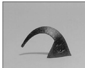
A self-supporting cone fired to maturity. Do not be concerned if the tip is slightly higher or lower than shown.
