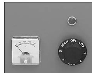
The pilot light serves as the pointer mark for the infinite control switch knob. The pyrometer shows temperature.
