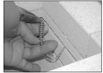
Bending the element at the corner. Use a screwdriver or pliers to hold the element while you pull it.
