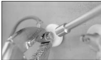
Hold the element connector with locking pliers when removing and installing the connector.
