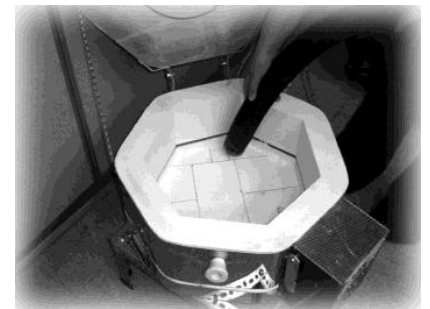
Vacuum any loose debris.
