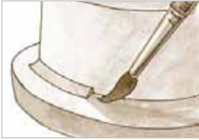
Use slip to fill between elements.
