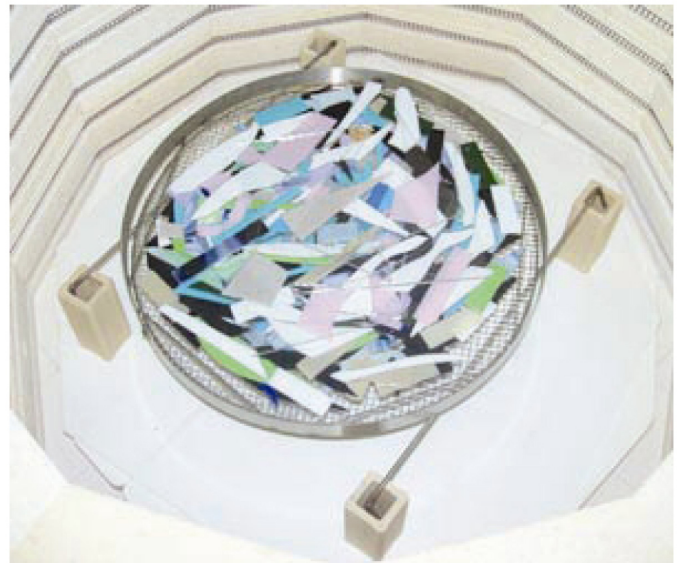
Screen melt and supporting ring standing on steel rod support bars standing on kiln posts.
