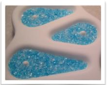
Fill each cavity according to the chart below. Rather than filling the mold evenly, best results can be obtained by slightly tapering the frit's level in the design. The frit should be "deeper" in the rounded portion of the design.
