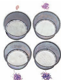
Separate frit of multiple grits using the 4 different mesh sizes.
