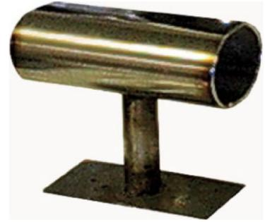
To push the ends of the napkin ring up and under the mandrel, gently rotate to the right and continue gliding along the surface of the glass until you have reached the right end of the glass. The handle of the tongs should nearly be touching the collar of the kiln when you have completed this motion to ensure you have a secure wrap. Repeat the same motion and gently rotate the tongs to the left and push the left end of the glass up under the mandrel.
