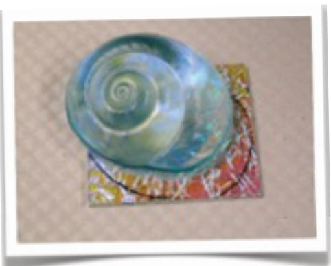
Remove all the kiln primer from the mold and reapply new Hotline Primo Primer™. Place the casting into mold and top it with the dichroic glass piece.
