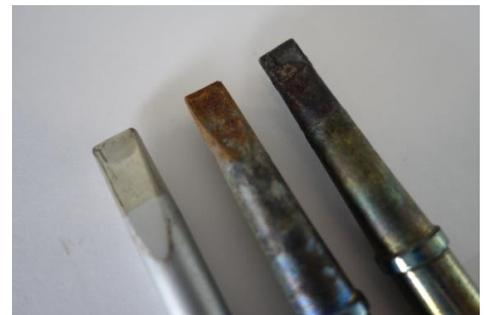
An oxidized tip can appear red or black like the tip in the middle and right. The tip on the left is clean.
