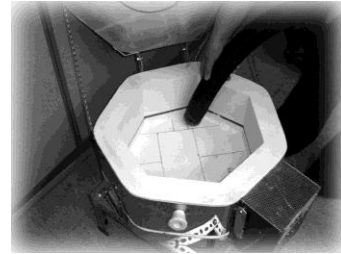
Vacuum any loose debris
