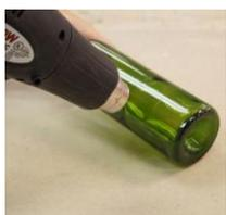
2. Run your score. We heated the bottle with a heat gun then used cold water and an ice cube to run the score.
